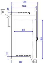
Electrical inlet (power) ΕI Refrigerant Outlet
